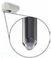
**Conical:** Conical, or spherical, is the most common and least expensive stylus type. It looks a bit like the tip of a ballpoint pen up close. Because of their relatively large radius, spherical styli trace less of the smaller groove modulations that represent higher frequencies.
