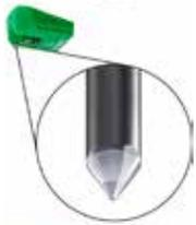
**Elliptical:** The next most common stylus type is elliptical, or bi-radial. Elliptical makes contact across a larger area of the groove wall due to its dual radii. This allows for more precise tracking, improved frequency response (especially highs), improved phase response, and lower distortion.
